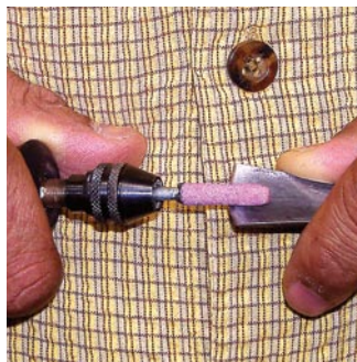
A Dremel tool can be used to shape the bevels on the inside edge of carving gouges.
