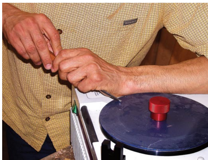
The Lap-Sharp has a large flat area next to the wheel. This allows sharpening with the hands in a natural carving position.
