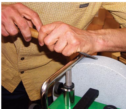
The best way to grind a good edge is with the hands as close as possible to the position they will be in when carving.
