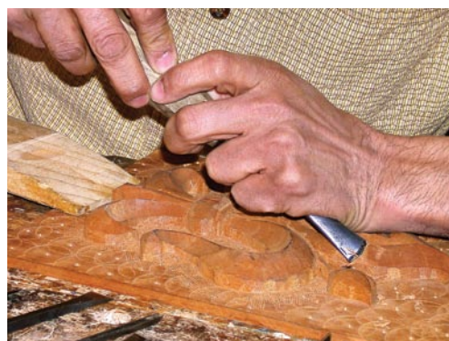
The bevel on the inside of the tool creates another shoulder, allowing the tool to cut both concave and convex shapes.
