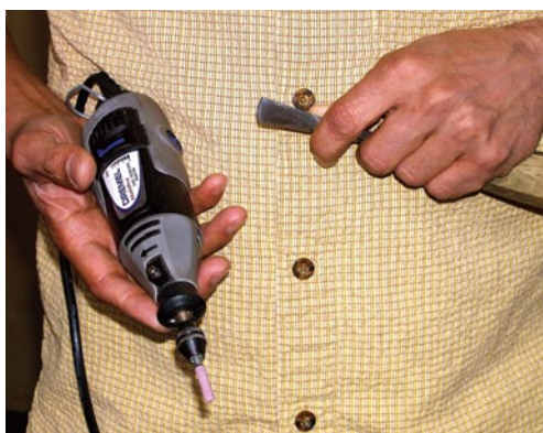
Holding the Dremel against the body allows the wrists to control both the tool and the grinder.
