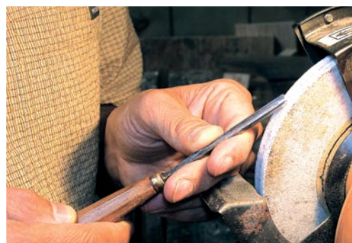
On a bench grinder, the left hand acts as a jig, so the tool can be returned to the same position after visual inspection.
