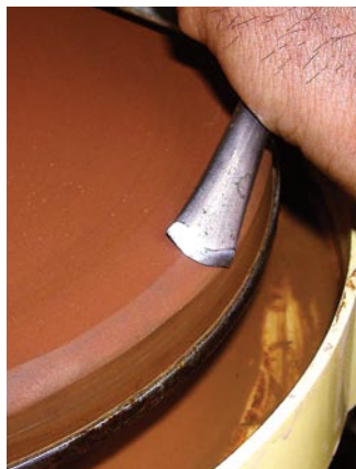
The outer edge of the waterstone can also be used to shape the inside bevel on larger tools.
